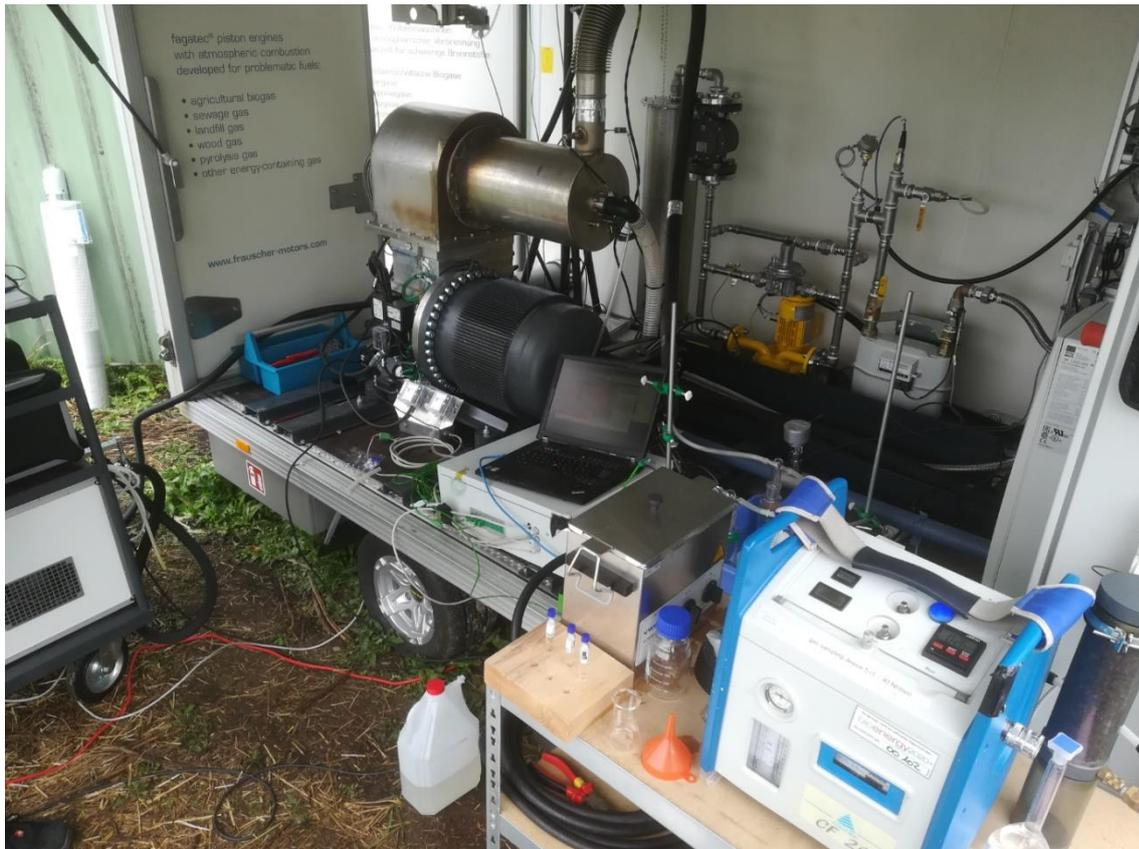
Figure 2: Measurement setup and Stirling cogeneration unit in the trailer.
