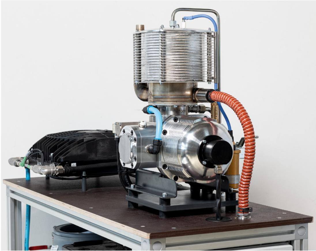
**FIGURE 2** First prototype of the unit with cooler heat exchanger
