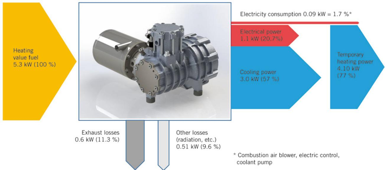
FIGURE 4 Overall energy balance (© Frauscher)
