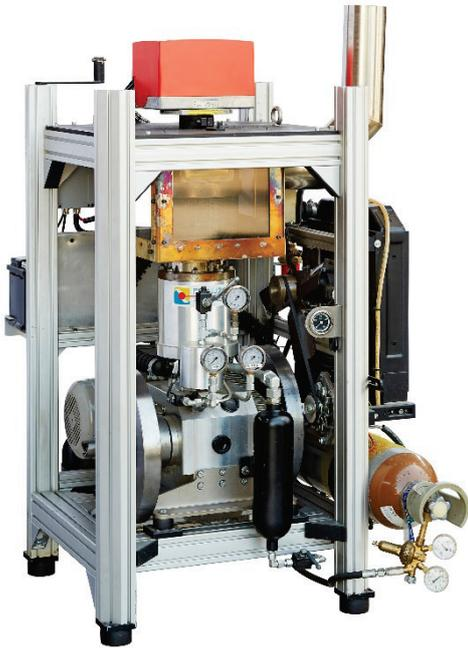
Figure 2: 250 cc Beta machine with rhombic drive
