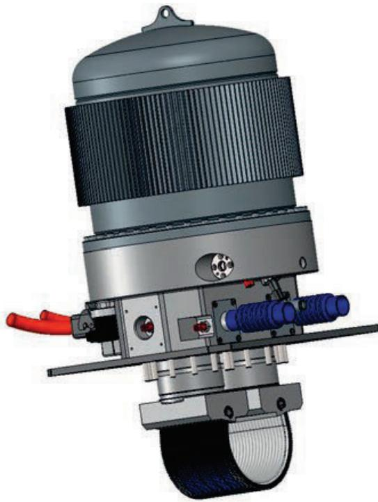
Figure 3: Type-A600 Stirling machine prototype
